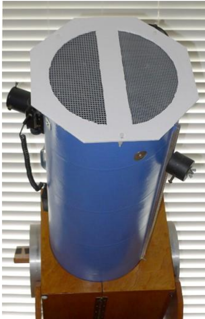
Figure 18. A 5-count coupled with a 7-count plastic mesh focusing mask on a 10-inch Newtonian in the Oleshko configuration.
