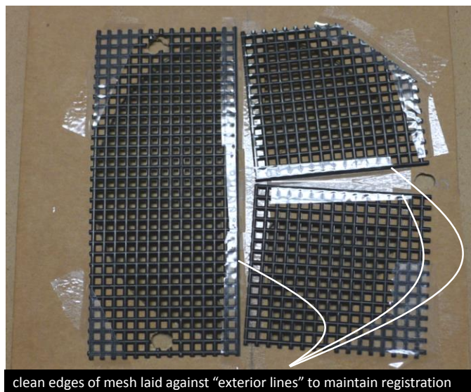
Figure 15. (L) Cutting out the holes. (R) The underside of the mesh Bahtinov.
