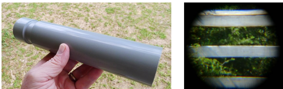
Figure A-7. The Dutch spyglass. The white-painted fence spans about a 3 degree real and a 9 degree apparent angle. Some chromatic aberration is visible, but I tend to seek the sweet spot near the center and aim the telescope accordingly.
