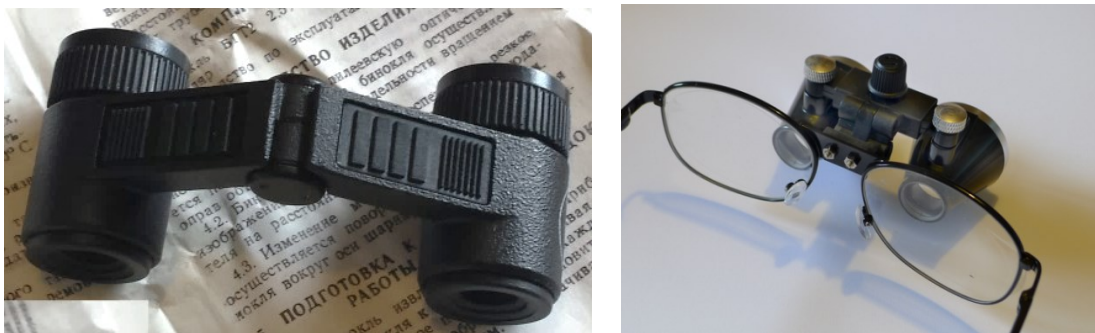
Figure 1. (left) A Russian miniature Galilean field glass: 2.5x17.5mm. (right) Medical Galilean eye loupe (~3x) focused at 320 mm
