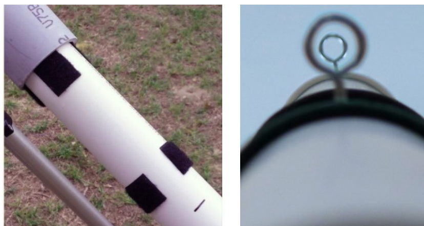
Figure 12. (left) Velcro felt tabs on withdrawn lower tube that allow smooth focusing. Insert tube to felt-tip mark to achieve distant focus. (right) Finder is a set of cup rings.
