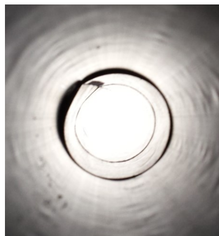
Figure 9. Interior of tube after papering upper end. The sloppy fit improves the baffling, so it was tolerated. (Aperture stop and lens not installed yet.)
