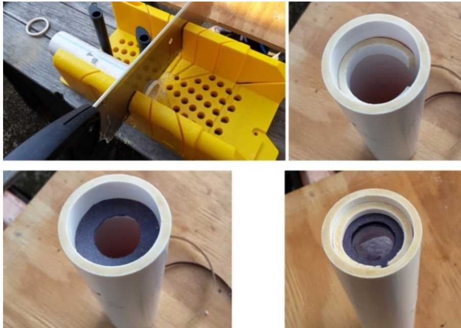
Figure 10. Assembly of a "lower" tailpiece or eyepiece end. The "upper" end is similar and not shown.
